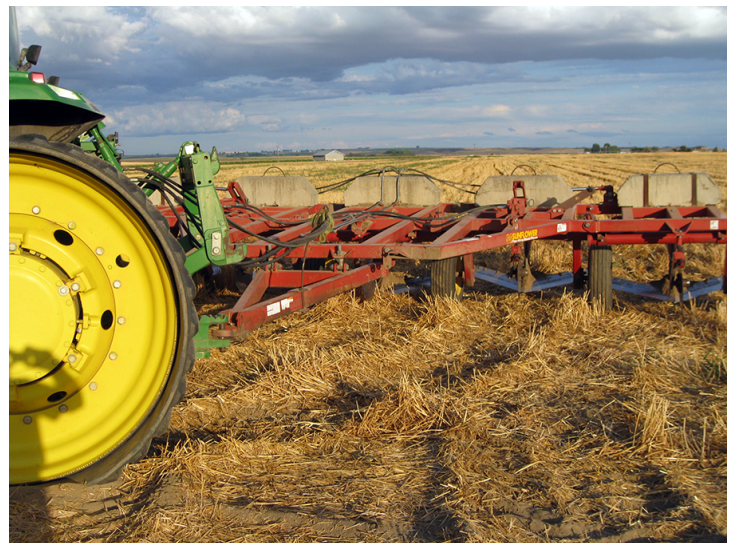
Figure 6. The undercutter Gies uses has 5.5-foot blades that are 5 feet apart. Gies operates the undercutter roughly 2–3 inches below the soil surface. Photo: Dale Gies.
